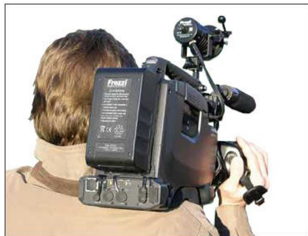
240WH Battery Powering Camera and Frezzi Dimmer Light
